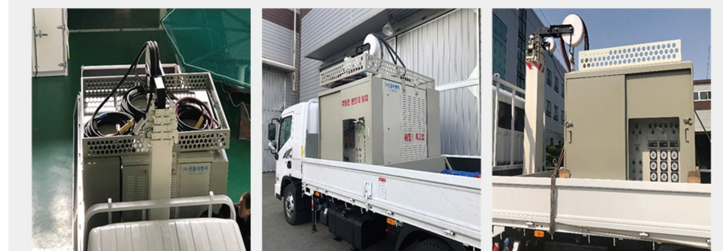
3.5Ton Truck Mounted Transformer Unit &amp; Boom Lift
